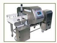
Overcome the limitations of fixed single or dual frequency metal detectors with the Thermo Scientific Sentinel Multiscan Metal Detector. By scanning up to five user-selectable frequencies running at a time, the Sentinel provides unmatched sensitivity and the highest probability of finding ferrous, non-ferrous and stainless steel metal contaminants in challenging applications such as dairy, meat, poultry, bread and other applications with high product effect.
