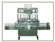
Used for small volume, accurate fills of ultra-clean or high-value liquids such as reagents, essential oils, pharma preparations and other applications where no cross contamination is permitted. Only low viscosity liquids can be used on this machine. The fluid path is disposable making cleanup very fast and efficient.
