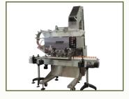
The SK6000X-BF6 is a fully automatic, inline, six spindle capper featuring an innovative belt feed system that eliminates vibratory bowls, overhead hopper loading and time consuming changeovers on a range of flat caps.
