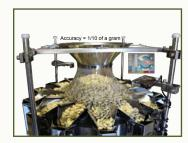
Combination Weighers and Counters are perfect for a wide array of high accuracy and high speed weighing and counting applications. They are easy to operate, clean and maintain. These systems will weigh/count your product and fill your containers with speeds up to 30-40 per minute and accuracies to a fraction of a gram. We are technology leaders in performance and reliability.
